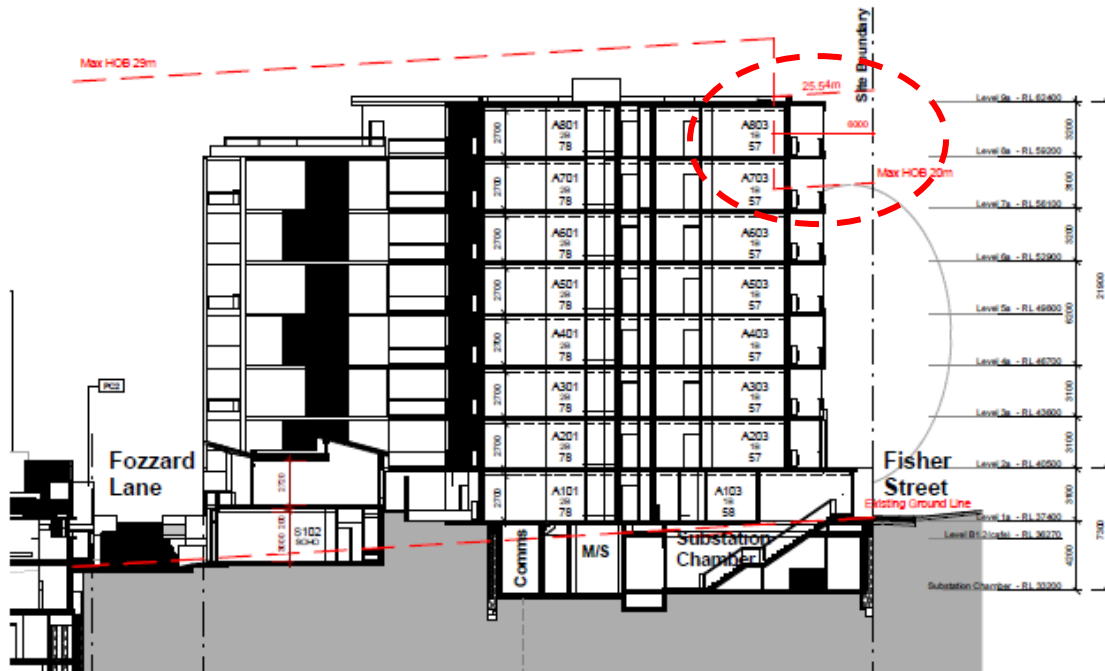
Figure 5: Extract of Section L for Building A in Site 3, variance (5.54 metres) circled in red (Source: Nordon Jago Architects)
